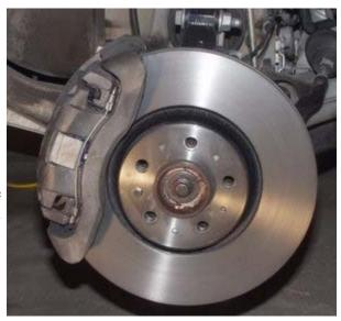
Repeat for the other side and enjoy!! Make sure to check your brake fluid before you are done. I bought my parts from Brentwood Volvo and Pads and rotors were ~\$160.00. I did "bed" the new pads with several repeated stops from about 50mph with time inbetween to cool.
