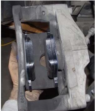
Pad orientation in caliper.
