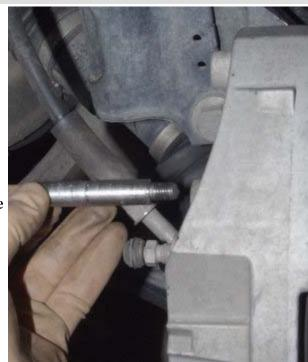
Remove old pads, finish compressing piston and suspend caliper safely with wire.
